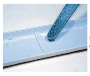
Sand inside lip of casting for easier fit over Walthers interior wall on car.
